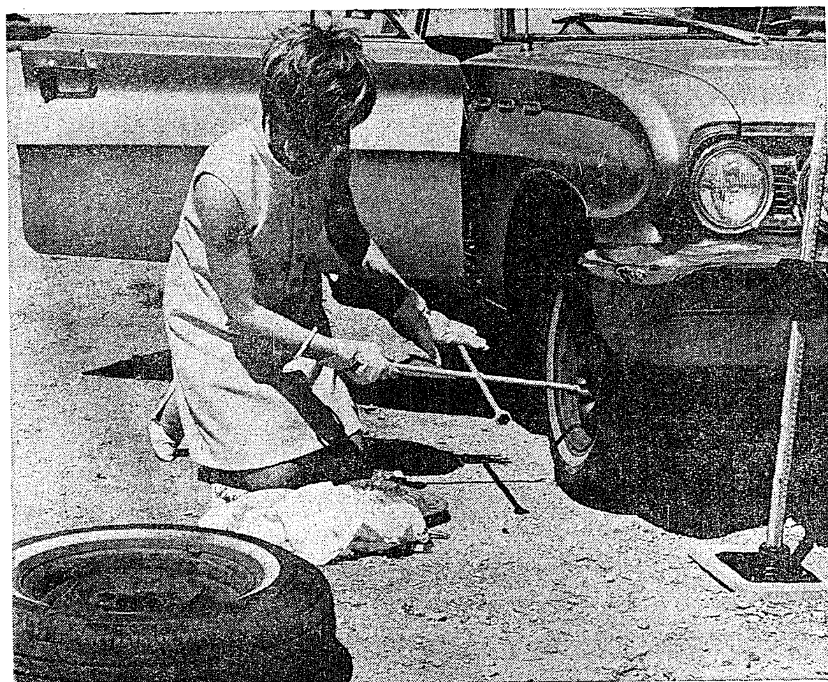
After jacking the car up, she removes the lug nuts.
